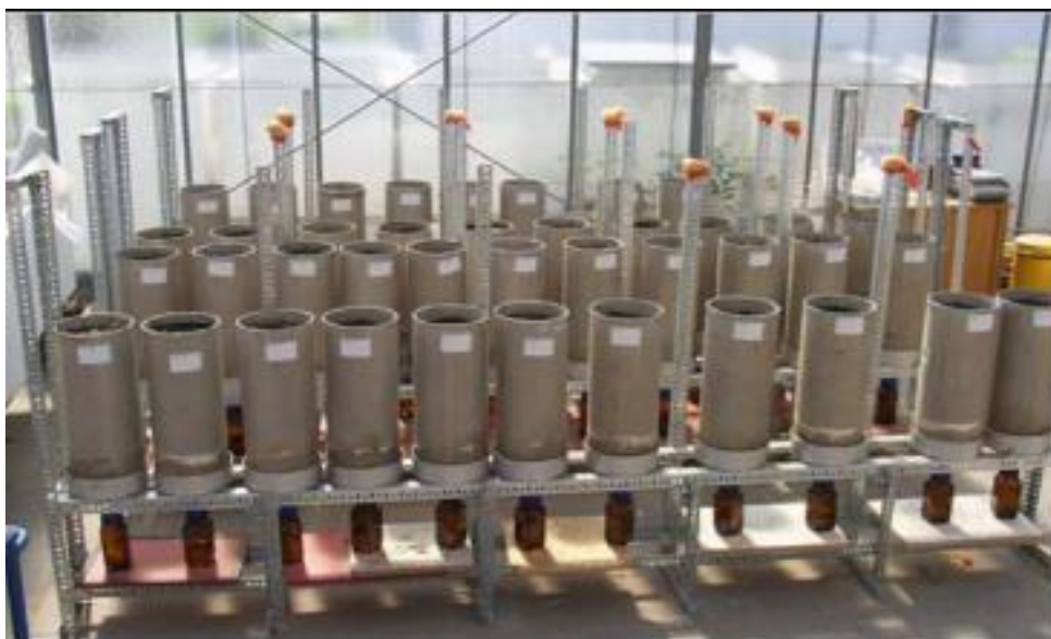
Figure 2.4. Soil column setup in a rack with several soil columns, column bases and brown glass bottles for leachate collection. Photo: Fabian Suttner.
